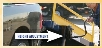
The two speed adjustable legs make height adjustment fast and easy.
