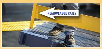
The hand rails improve operator safety and are removable when needed.
